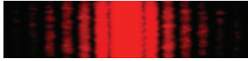
Figure 37.1 The diffraction pattern that appears on a screen when light passes through a narrow vertical slit. The pattern consists of a broad central fringe and a series of less intense and narrower side fringes.
