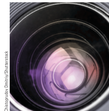
Figure 36.12 (Example 36.4) (a) Reflective losses from a silicon solar cell are minimized by coating the surface of the cell with a thin film of silicon monoxide. (b) The reflected light from a coated camera lens often has a reddish-violet appearance.
