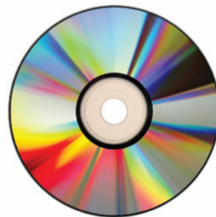
Figure 37.14 (Conceptual Example 37.4) A video disc observed under white light. The colors observed in the reflected light and their intensities depend on the orientation of the DVD relative to the eye and relative to the light source.
