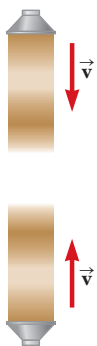
Figure 17.6 Two identical loudspeakers emit sound waves toward each other. When they overlap, identical waves traveling in opposite directions will combine to form standing waves.
