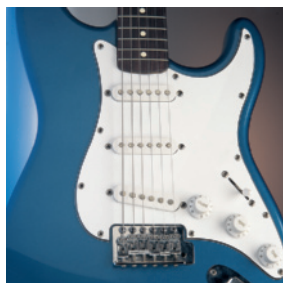
Figure 30.5 (a) In an electric guitar, a vibrating magnetized string induces an emf in a pickup coil. (b) The pickups (the circles beneath the metallic strings) of this electric guitar detect the vibrations of the strings and send this information through an amplifier and into speakers. (A switch on the guitar allows the musician to select which set of six pickups is used.)
