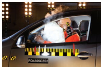
Figure 9.4 A crash-test dummy is brought to rest by an air bag in a test collision. The air bag increases the time interval during which the dummy is brought to rest, thereby decreasing the force on the dummy. Air bags in automobiles have saved countless human lives in accidents.
