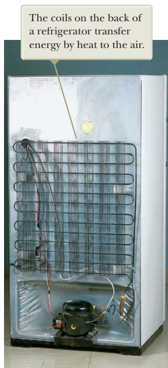
Figure 21.6 The back of a household refrigerator. The air surrounding the coils is the hot reservoir.
