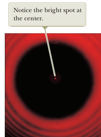
Figure 37.3 Diffraction pattern created by the illumination of a penny with a laser, with the penny positioned midway between the screen and laser.
