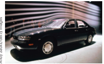
Figure 14.13 Laminar flow of smoke over an automobile in a test wind tunnel.
