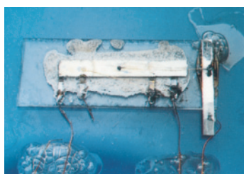
Figure 42.30 Jack Kilby's first integrated circuit, tested on September 12, 1958.
