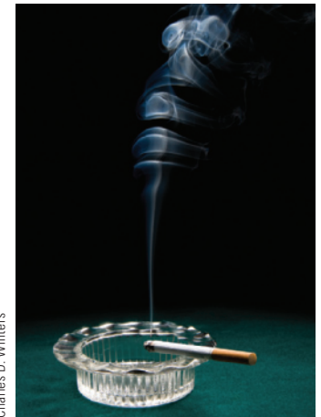
Figure 14.14 Hot gases from a cigarette made visible by smoke particles. The smoke first moves in laminar flow at the bottom and then in turbulent flow above.
