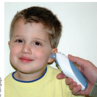
Figure 39.8 An ear thermometer measures a patient's temperature by detecting the intensity of infrared radiation leaving the eardrum.
