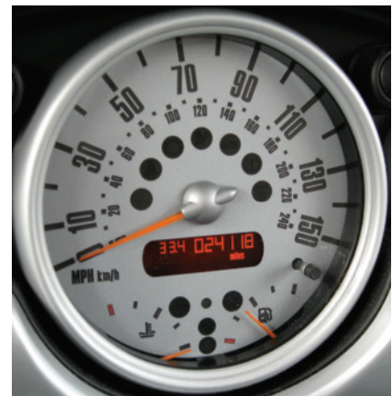
Figure 1.6 The speedometer of a vehicle that shows speeds in both miles per hour and kilometers per hour.
