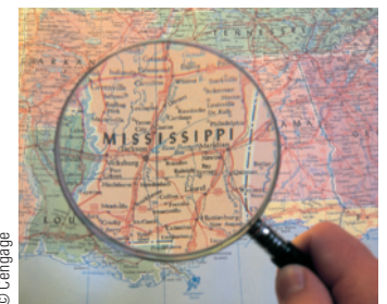
Figure 35.42 A simple magnifier, also called a magnifying glass, is used to view an enlarged image of a portion of a map.
