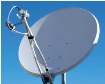
Figure 35.10 A satellite-dish antenna is a concave reflector for television signals from a satellite in orbit around the Earth. Because the satellite is so far away, the signals are carried by microwaves that are parallel when they arrive at the dish. These waves reflect from the dish and are focused on the receiver.
